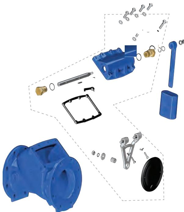
To achieve the optimum performance from any swing check valve, a velocity of 1.5 to 2m/s is required to fully open the valve, and to reduce turbulence a straight piece of pipe five (5) times
