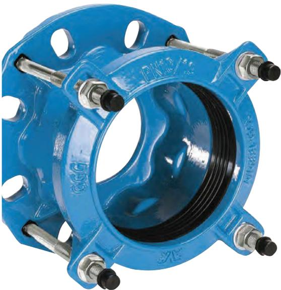
The AVK Supa® universal straight couplings, step couplings and flange adaptors are suitable for uPVC, cast iron, ductile iron, steel and AC pipes. The couplings range from DN40 to 400 and are suitable for water and wastewater applications.
