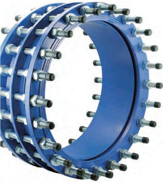
AVK fabricated dismantling joints provide easy installation and disassembly of flanged pipework and equipment and compensate for axial displacement of the pipe during installation and dismantling. The range is available in DN80-2000 in PN10/16 and up to DN1200 in PN25.
