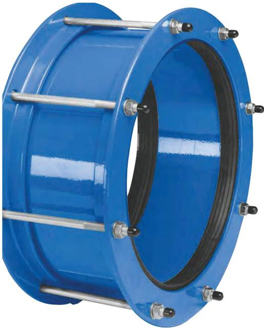
AVK's range of fabricated fittings comprises non-tensile straight couplings, step couplings and flange adaptors in DN80-2000. The range is suitable for ductile and grey cast iron, steel, uPVC and GRP pipes for water applications up to 25 bar.
