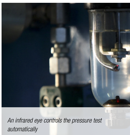
Every single valve is pressure tested
