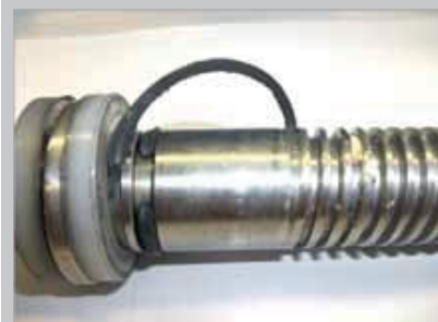
Damaged spindle thread and O-ring
