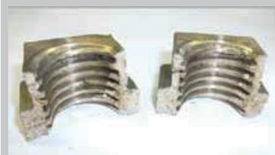
Broken wedge nut
