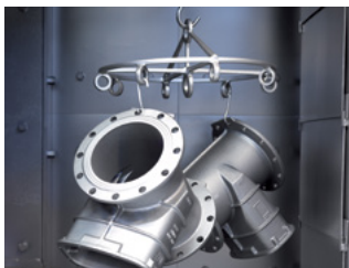
AVK valves are blast-cleaned according to ISO 12944-4
