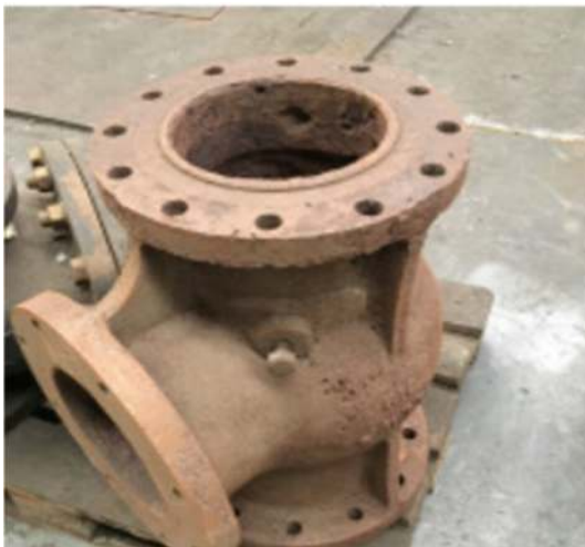
Original cast body after shot blasting
