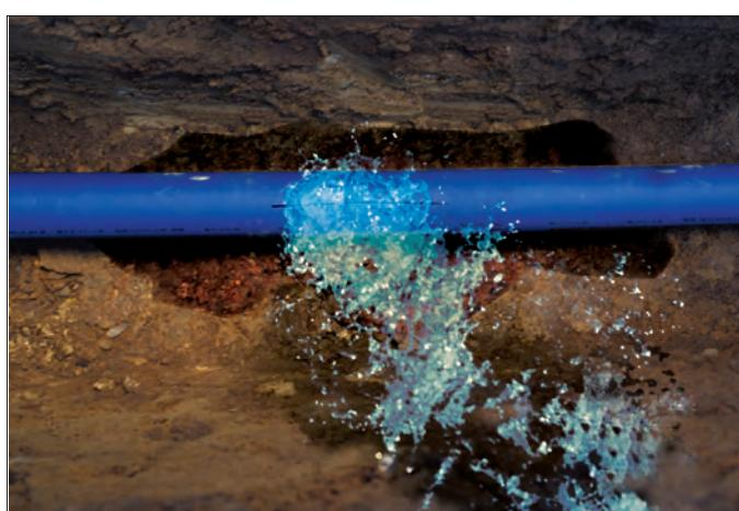
Typical longitudinal crack in a pipe typically caused by earth settlement or increased traffic load.
