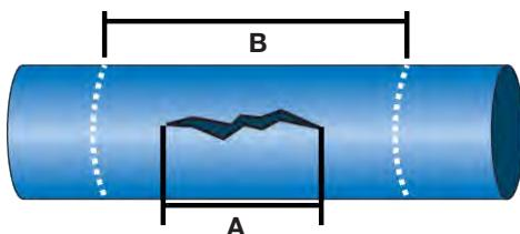
Width of repair clamp, B, shall be at least 3 times of length of length of crack or hole, A.
