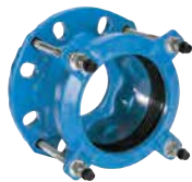
Series 603 Supa® flange adaptor universal for uPVC, AC, steel, cast iron and ductile iron pipes Universal drilling Ductile iron PN10/16
