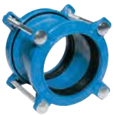
Series 601 Supa® straight coupling universal for uPVC, AC, steel, cast iron and ductile iron pipes Ductile iron PN16
