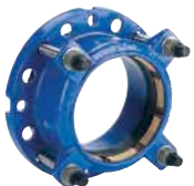
Series 623/10 Supa Plus™ flange adaptor Tensile for PE and uPVC pipes Universal drilling Ductile iron PN10/16
